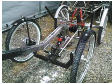
RIGHT: At both front and rear, the suspension system has single shared swing-arms for both wheels.
