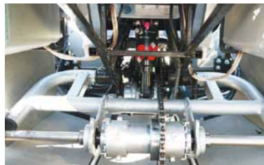
RIGHT: The transmission system is rather elaborate, with gearing systems both before and after the mid-mounted electric motor.
