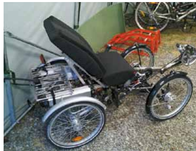
RIGHT: Two battery packs are fitted behind the seat, and there's space on top of them for luggage.
