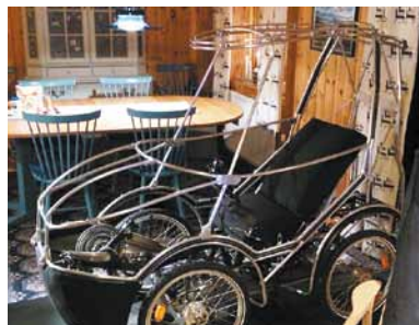
RIGHT: The aluminium framework for the fabric fairing is lightweight and easily adaptable to create different styles.
